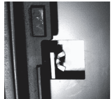
The wing nut that holds the front door is accessible through the cut-out in the right side heat shield.
